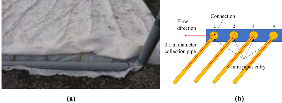
Fig. 5. Experimental set up to address singular head loss through connection between mini pipes and the header pipe for gas drainage facilities: (a) field set up and (b) experimental set up.
