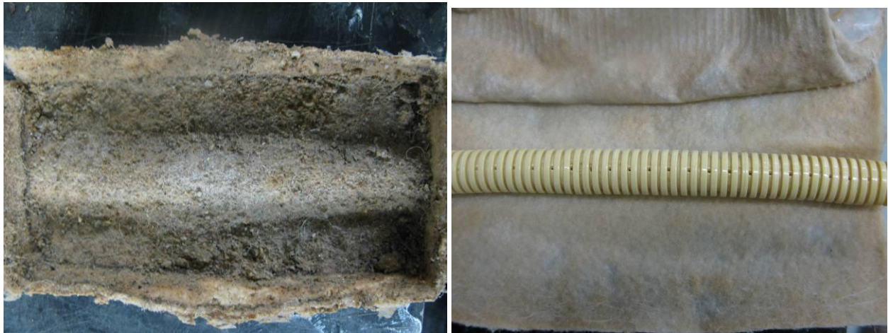
Figure 6: external and internal view of the geocomposite after 3 months of percolation of sulphuric acid
