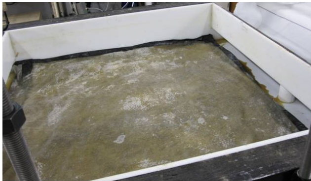
Figure 4 : 25mm layer of sand (confined in a thin plastic sheet) installed as a foundation layer in the LST
