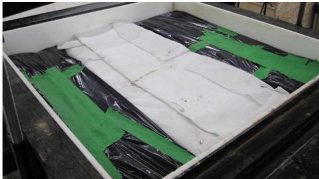
Figure 12 : 500 mm x 1000 mm specimen installed in the LST
