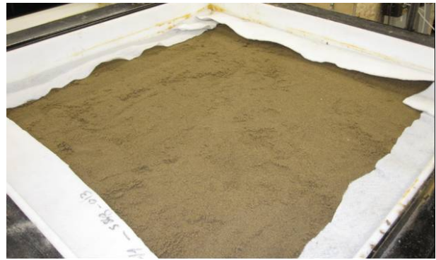
Figure 5 : Daintube covered by sand. The cover geotextile was wrapped around the sand to contain it
