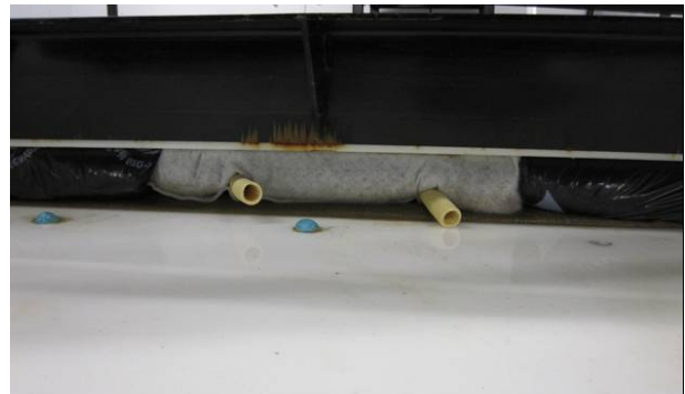
Figure 13 : 500 mm x 1000 mm specimen with 2 x 25mm pipes installed in the LST
