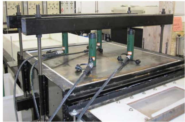
Figure 2 : Loading mechanism (load distribution layer not shown)
