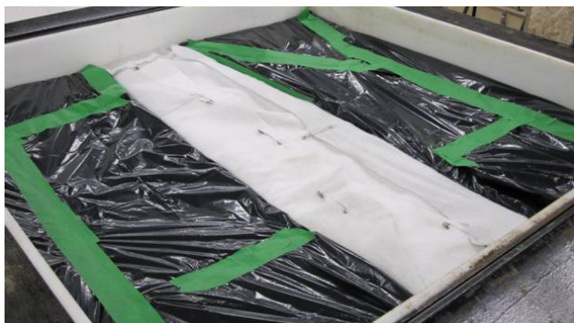
Figure 14 : 250 mm x 1000 mm specimen installed in the LST
