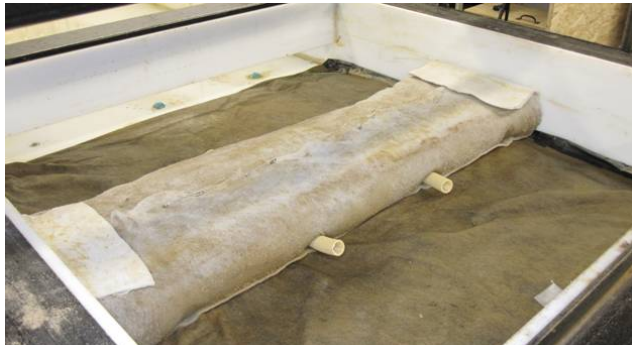
Figure 10 : 1000 mm x 250 mm specimen with 2 x 25mm pipes installed in the LST
