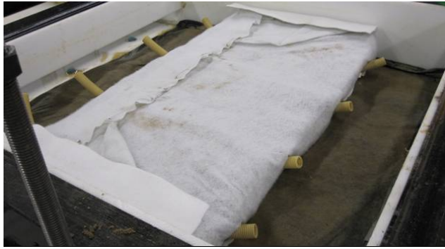
Figure 8 : 1000 mm x 500 mm specimen installed in the LST
