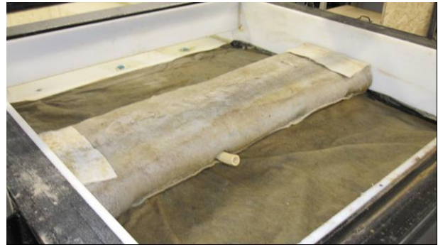
Figure 11 : 1000 mm x 250 mm specimen with 1 x 25mm pipe installed in the LST
