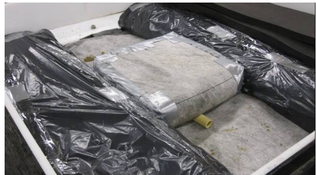
Figure 7 : 250 mm x 300 mm specimen installed in the LST
