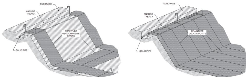
**Fig. 6.** Installation of the geocomposite on partial-surface or full-surface.
