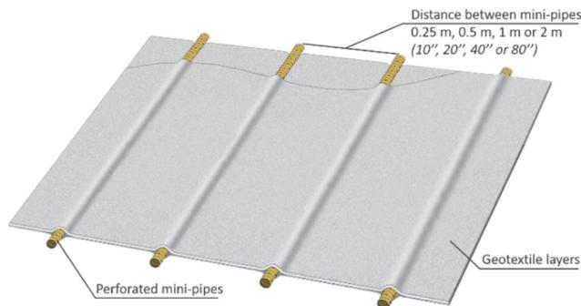
**Fig. 1.** Draintube geocomposite description.
