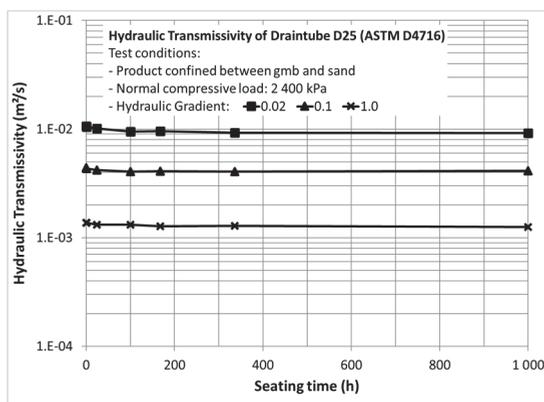
**Fig. 3.** Hydraulic transmissivity of the DRAINTUBE multi-linear drainage geocomposite under load and over time.
