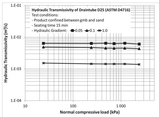
**Fig. 2.** Hydraulic transmissivity of the DRAINTUBE multi-linear drainage geocomposite for several loads.
