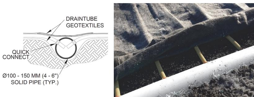
**Fig. 4 & 5.** Connection using the quick connect system.
