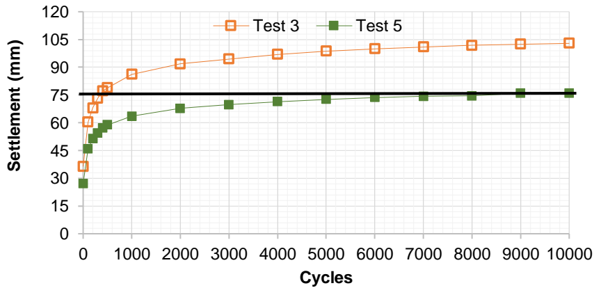
Figure 4: The settlement evolution with cycles at the base course surface centre for H=22cm.
