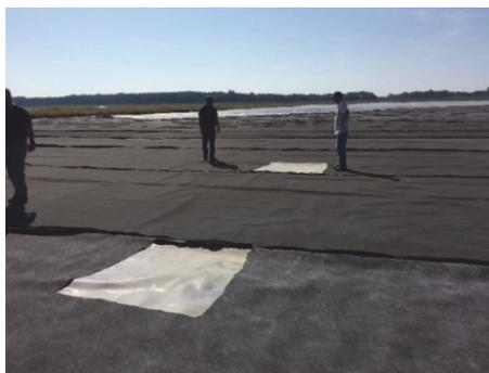
**Fig. 7.** Photo of geotextile being sampled.
