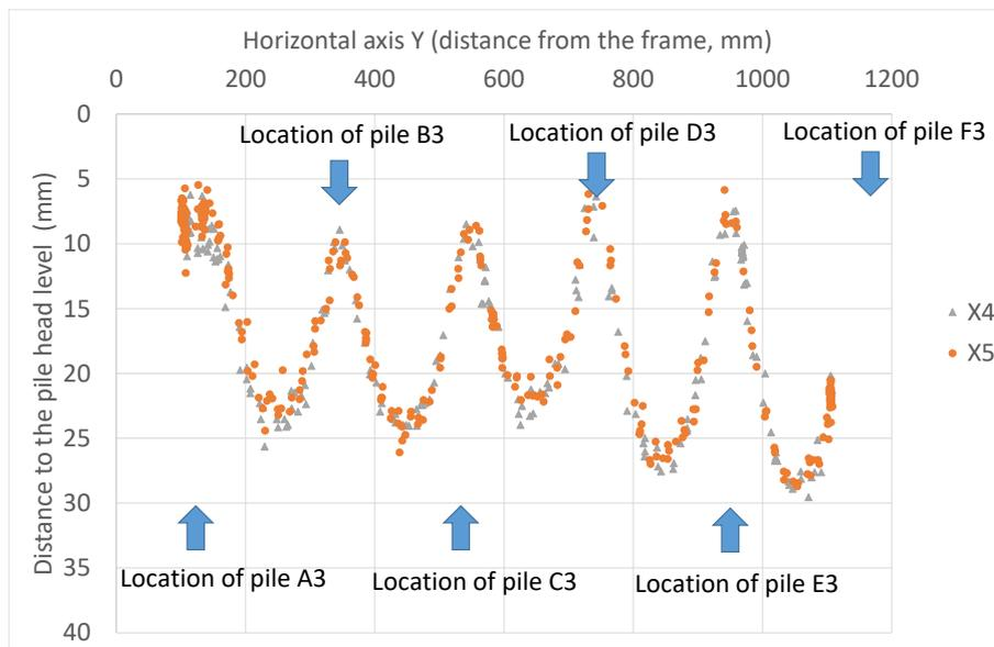
Figure 7. Deflection of the geosynthetic under a layer of 20 cm of sand
