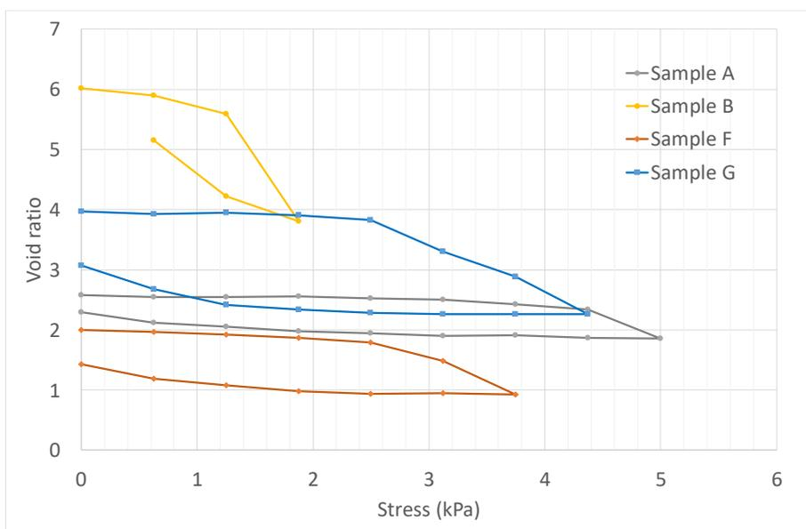
Figure 5. Compressibility tests
