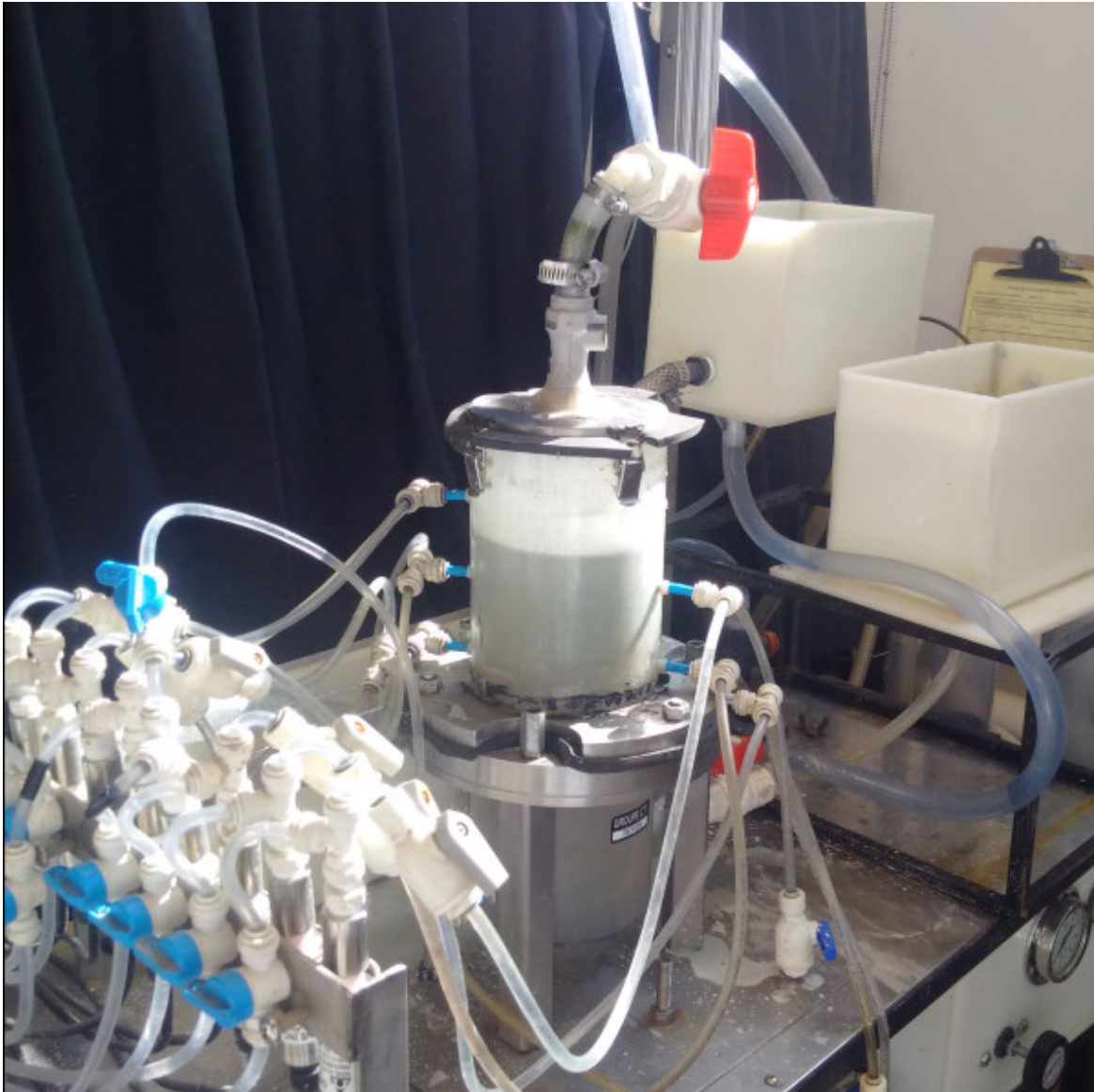
Figure 7 Set-up of the filtration test (Gradient Ratio, ASTM D5101)
