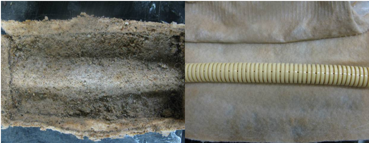
Figure 4 External and internal view of the geocomposite after 3 months of percolation of sulphuric acid
