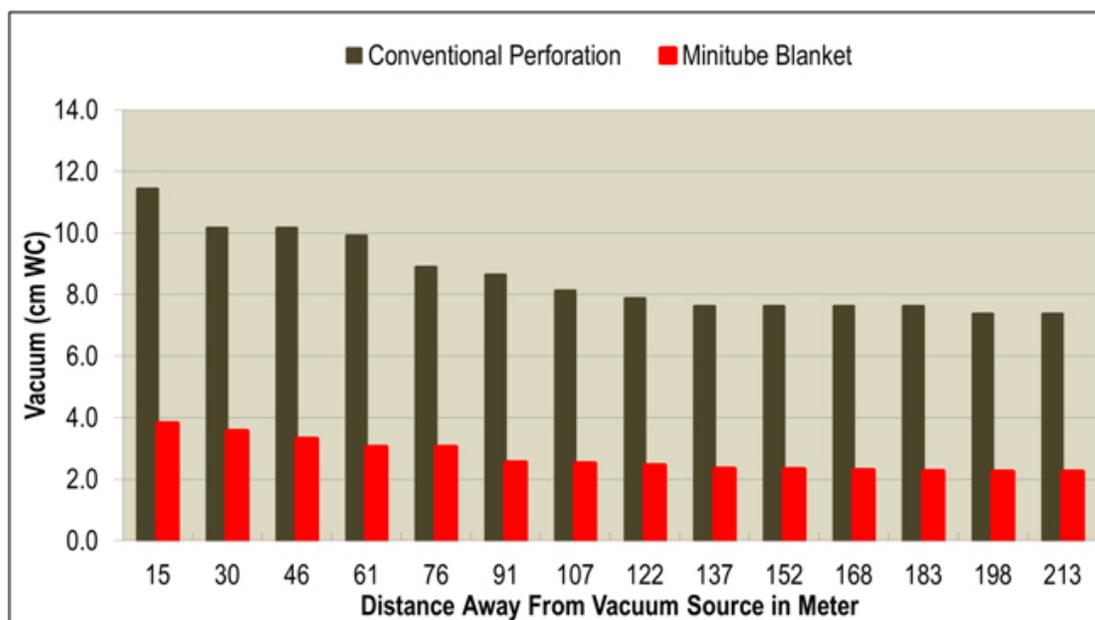
**Figure 5: Vacuum dissipation along trench.**
